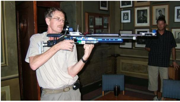
This is an Air Rifle manufactured by the company Feinwerkbau. It is the standard of rifle used in the Olympic Games, for the indoor 10m range. These rifles fire pellets, and are operated using compressed air. The pressure is around 150 - 180 bar. A charged cylinder is capable of firing about 40 - 60 shots before the pressure difference starts affecting accuracy.
